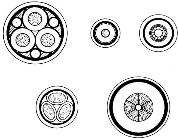
**Figure 31.15** Cross-sections of typical oil filled cables
