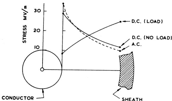
**Figure 31.18** Stress distribution in d.c. and a.c. cables
