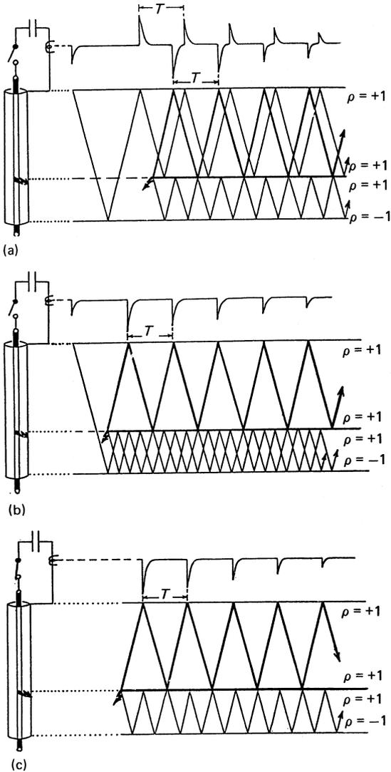
**Figure 31.30** Current transients created by the application of an impulse voltage from a charged capacitor: (a) voltage doubling induced breakdown; (b) fault breakdown before reflected pulse; (c) simpler transient produced by closing the generator contactor
