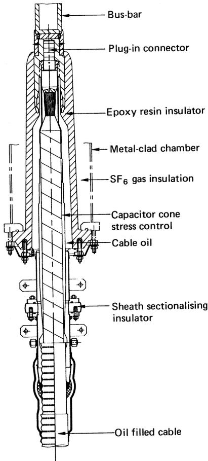
Figure 31.27 SF<sub>6</sub> plug-in sealing end for 132 kV OF cable
