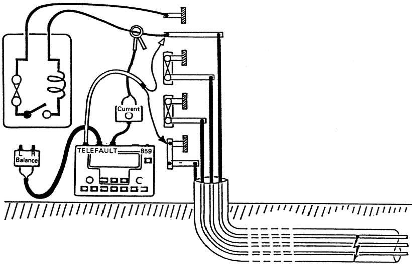
Figure 31.34 Test lead connected to the cable termination
