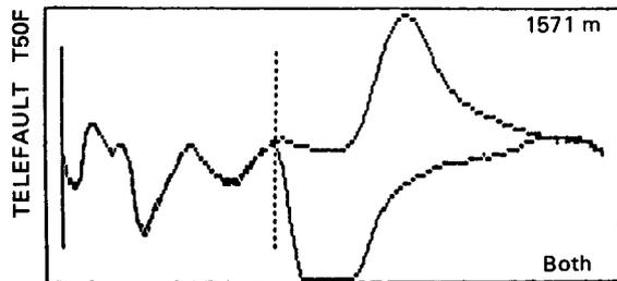
Figure 31.35 Typical secondary impulse method result
