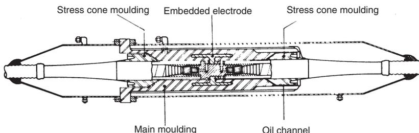
**Figure 31.26** Single-core, 132 kV, OF cable stop joint
