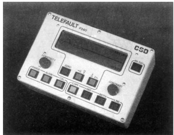
**Figure 31.33** Digital pulse echo instrument
