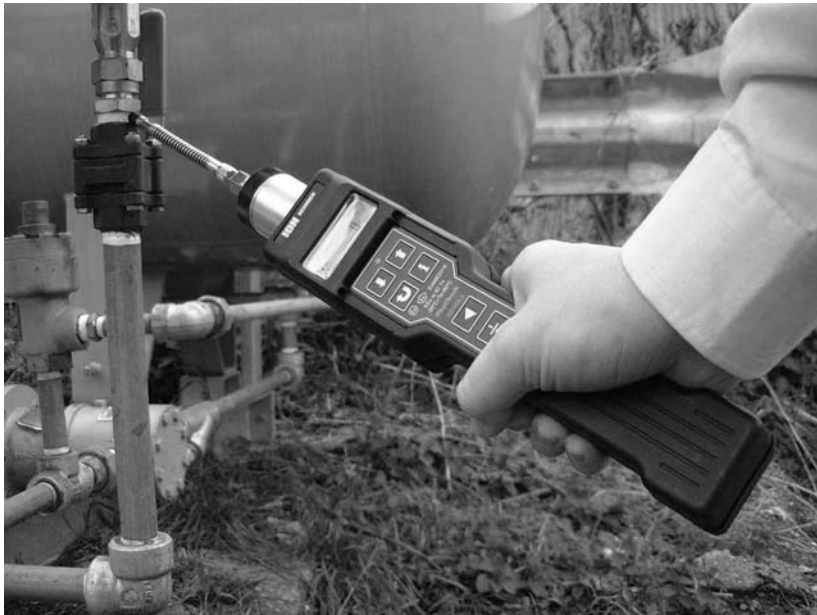
Figure 25.3 An example of a battery powered hand held intrinsically safe instrument. Photograph courtesy of Ion Science Ltd
