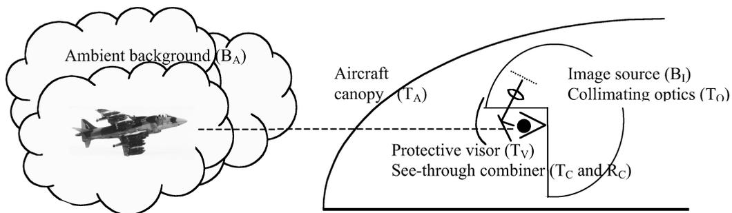
**FIGURE 5.15** Contributions for determining image source luminance requirements for an HMD in an aircraft cockpit.
