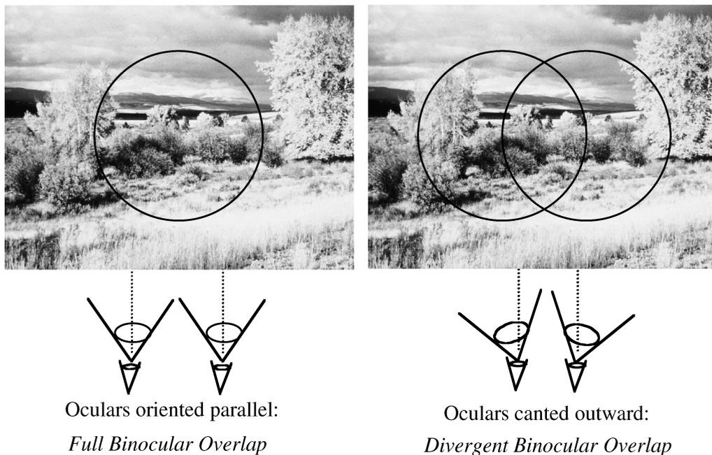
**FIGURE 5.14** Comparison of a full binocular overlap and divergent partial binocular overlap. Note the increase in viewable imagery in the horizontal direction with the divergent overlap.
