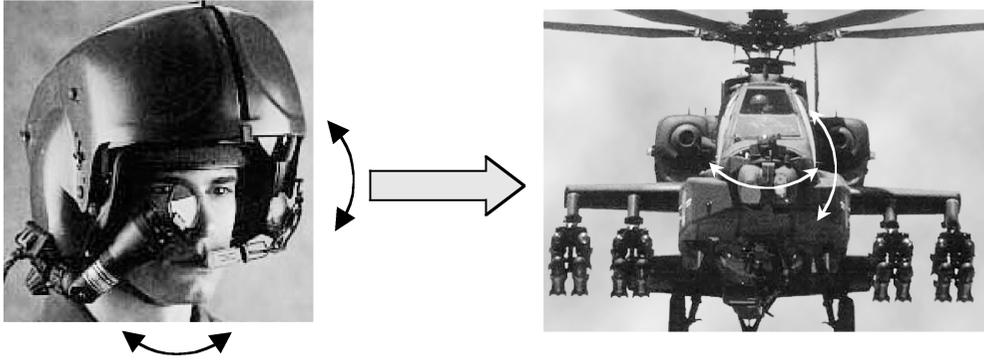
**FIGURE 5.11** The linkage between the IHADSS helmet-mounted display and the Pilot's Night Vision System in the AH-64 Apache helicopter. The PNVS is slaved to the pilot's head line of sight. As he turns his head, the PNVS turns to point in the same direction.
