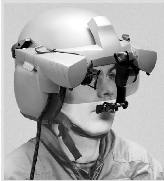
**FIGURE 5.4** A prototype of the Kaiser Electronics' HIDSS for the RAH-66 Comanche helicopter. (Photo courtesy of Kaiser Electronics, used with permission.)
