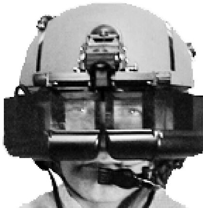
**FIGURE 5.13** Proview™ 100 HMD mounted on SPH-4B helicopter helmet for a simulator application. This is an example of an optically tiled see-through HMD with 100° by 30° field of view. (Photo courtesy of Kaiser Electro-Optics, used with permission.)
