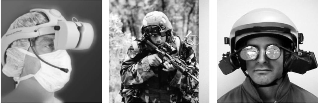
**FIGURE 5.1** Three different applications for HMDs: the CardioView® for minimally invasive cardiac surgery (photo courtesy of Vista Medical Technologies, Inc.), a prototype of the U.S. Army Land Warrior HMD (photo courtesy of Program Manager, Soldier, U.S. Army), and the SIM EYE XL100 for aviation training (photo courtesy of Kaiser Electro-Optics).
